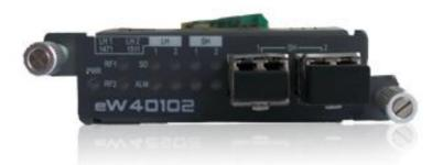
**eW40102 Series** is an dual channel 100M~1.25G multi-rate transponder card used in eWAVE4107 and eWAVE4214 platform. It provides a low cost solution, supports 2X1.25G transmission with 1 slot of eWAVE4107 or eWAVE4214. SFP modules are used in client side, which support 850nm, 1310nm or 1550nm according to different application. Line side ports are implemented by CWDM/DWDM SFP modules which support 40km, 80km, and 120km transmission.
